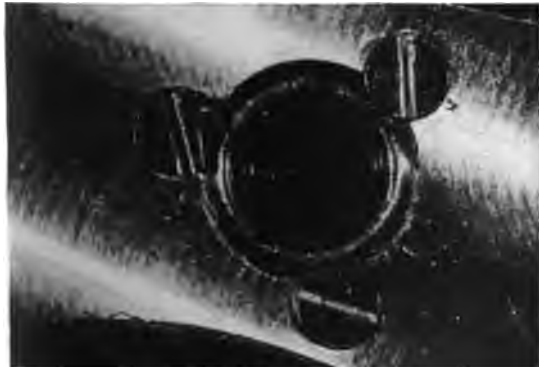
THREE TINY SCREWS HOLDING A SMALL JEWEL.
